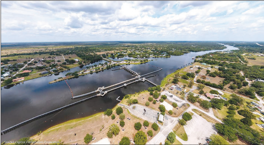
An aerial view of the Franklin Lock (designated S-79), the final U.S. Army Corps of Engineers water control structure between the Caloosahatchee and its interface with the estuary. The lock helps control water released from Lake Okeechobee. photo courtesy SCCF
